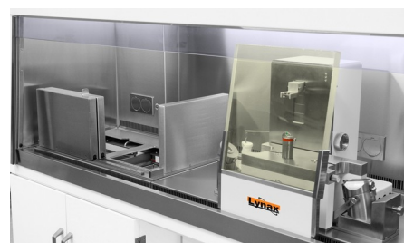
LWB18 PET/Ga working area with the PT459R5 dispensing unit
