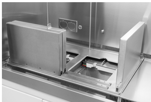
Configuration for 68 Ga generators – open compartment
